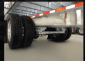
AANL-230 w/ 250 air bags & Hendrickson HXL-5 sealed Wheel End Sys. (5-yr. Warranty) Galv. suspension hangers & brace.
