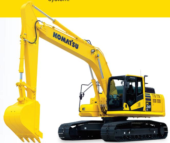
A powerful **Komatsu SAA6D107E-3 engine** provides a net output of 132 kW **177 HP**. This engine is EPA Tier 4 Final emissions certified.
