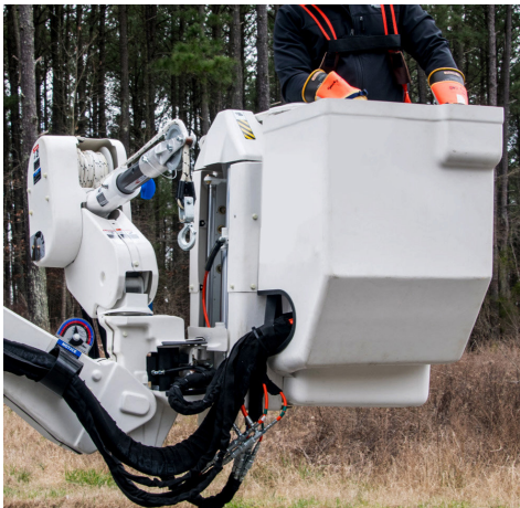
24" PLATFORM ELEVATOR OPTIMIZES OPERATOR REACH WITHIN WORK ZONE
