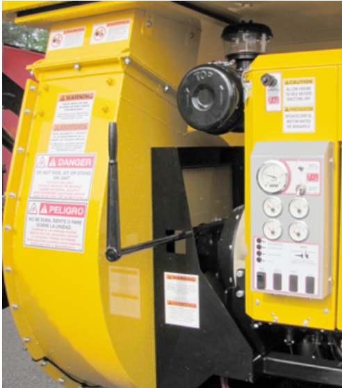
PTO shown fully engaged
