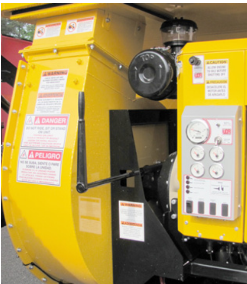
PTO shown fully engaged
